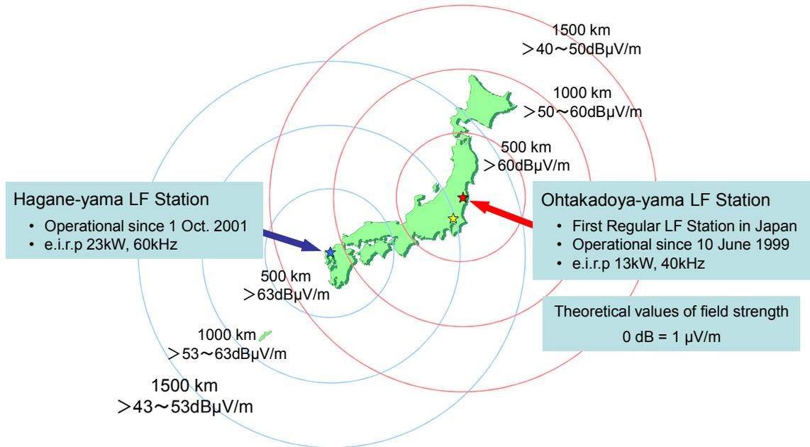
**Figure 1. LF time and frequency service in Japan. The values under the distance (km) shows the approximate strength calculated as the assumed electric field.**
