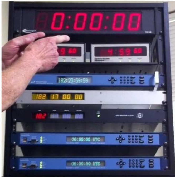
**Figure 5. Skip Newhall’s 2012 leap second party gear at 23:59:60. Only the WWVB receivers conform to TF.460**
