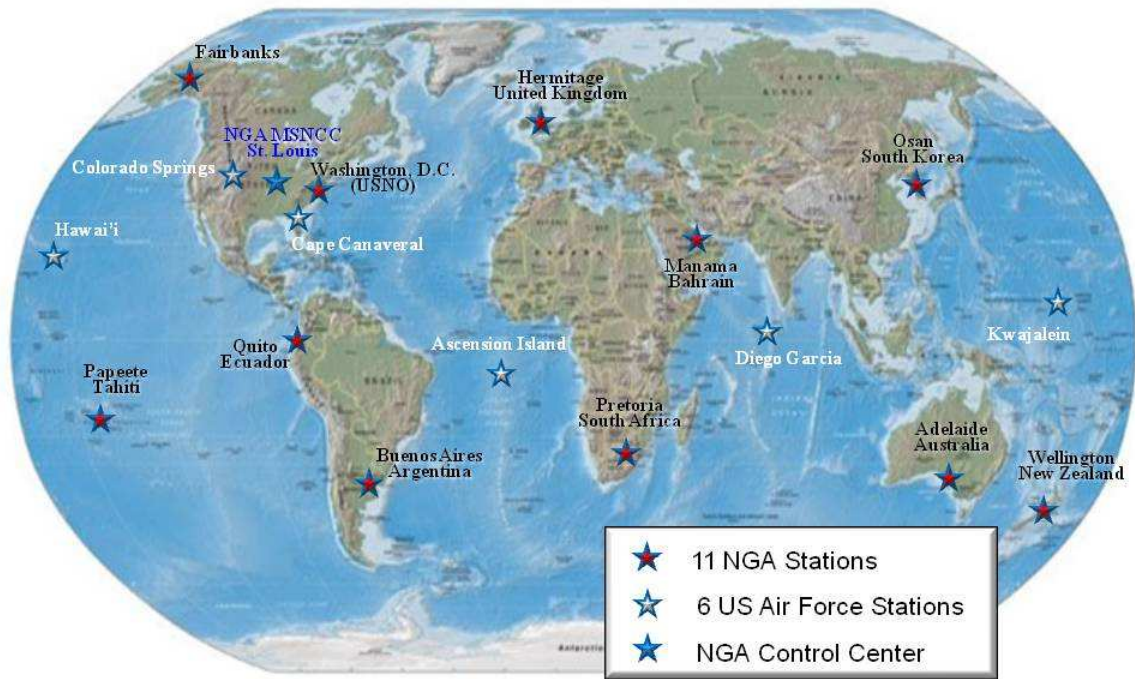
Figure 1. DoD GPS Monitor Station Network.
